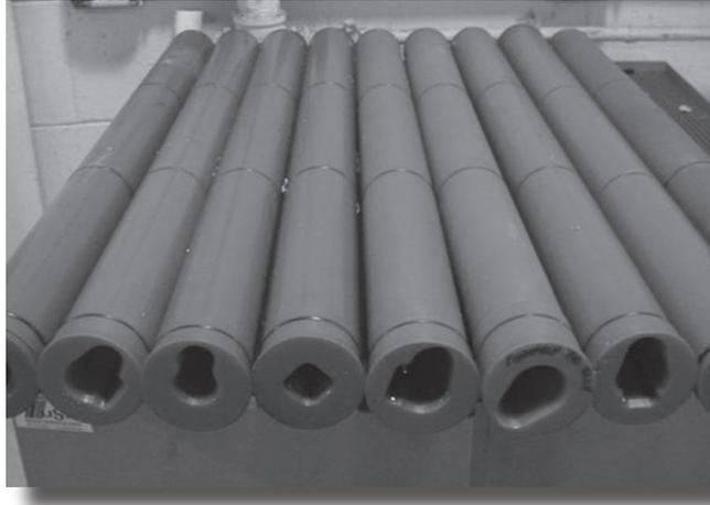
The spindle liners combined with shaped collets would allow what were once twin-operation machining center jobs to be run on the Eurotechs by stopping the machines and manually loading fresh bars at frequent intervals. It is the addition of a part feeder that can accommodate shaped bars that allows these parts to be finished in one
